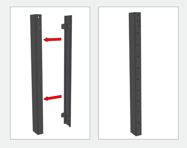
5. Connect the telescope pipe to the ceiling mount.
